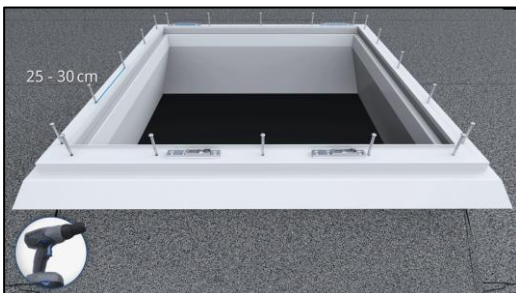
12 Multirahmen verschrauben Fix multi frame with screws
